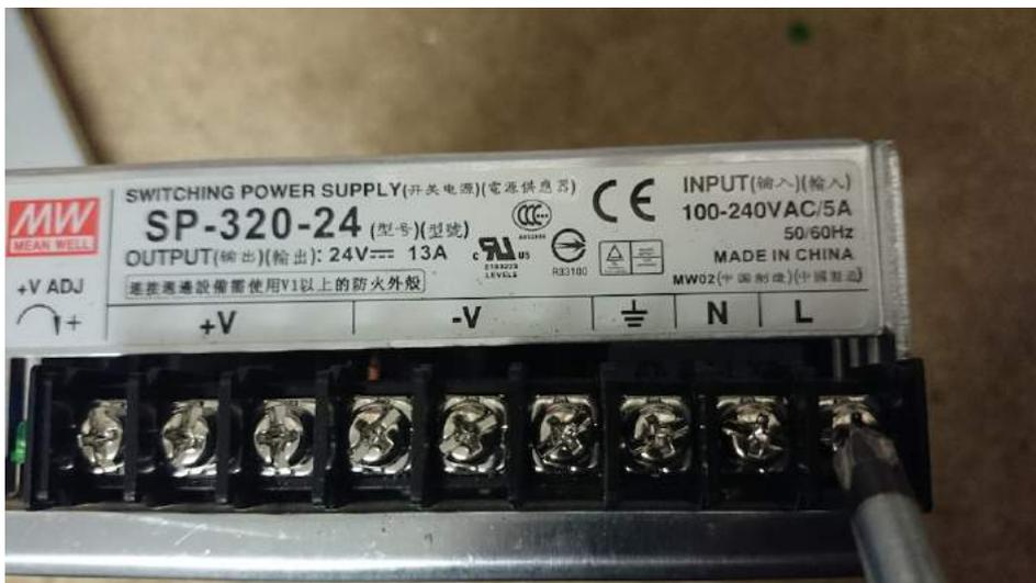
3. Take the 3-core power cable with plug, and connect each cable to the correct matching connection. The Brown cable should be wired to the L connection, and the Blue cable to the N connection. Finally, the Green/Yellow connects to the ground connection.
