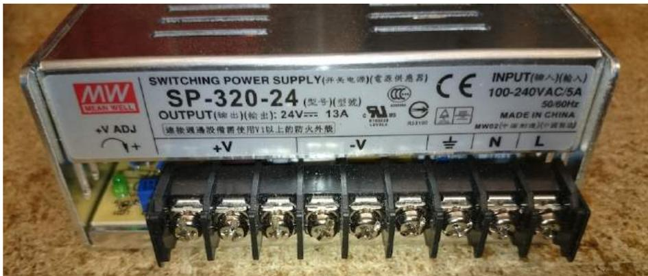
2. Unscrew the L, N, and ground connections.
