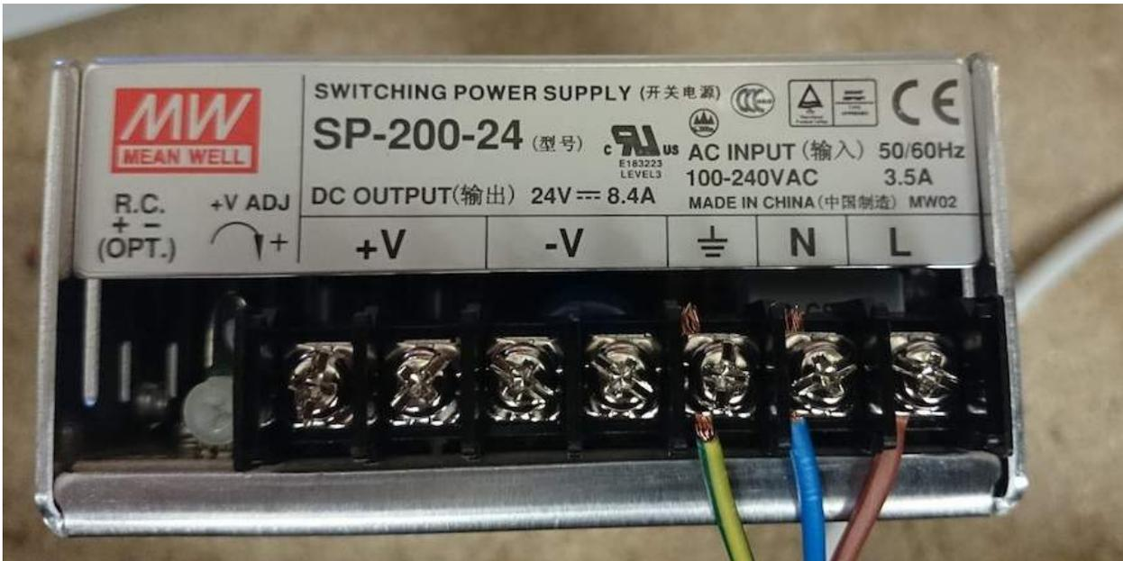
4. Now take the LED tape you intend to power, and connect each of its cables to the correct connection. With 2-core cable, you should connect the Red/Brown lead connects to '+' and the Black/Blue lead to '-'.
